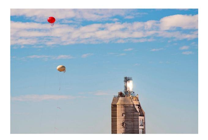
A team of researchers from Sandia National Laboratories recently used tethered balloons to collect samples of airborne dust particles to ensure the safety of a falling-particle receiver for concentrating solar power, an emerging solar power technology. Credit: Randy Montoya/Sandia National Laboratories
