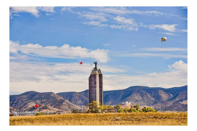
Three tethered balloons were deployed both upwind and downwind of Sandia National Laboratories' National Solar Thermal Test Facility during a fallingparticle receiver test. The team, led by Cliff Ho, found that the concentration of tiny particles, finer than talcum powder, that escape from the receiver were much lower than Environmental Protection Agency limits. Credit: Randy Montoya/Sandia National Laboratories
