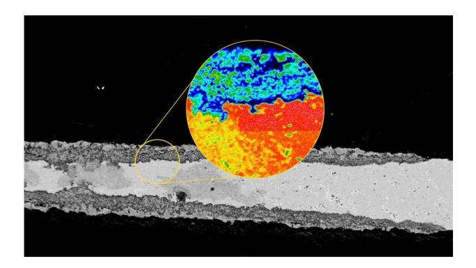
MAX phases material (an example shown in electron micrograph) are some of the most high-temperature corrosion and oxidation-resistant materials to date. Credit: Dr. Miladin Radovic/Texas A&M Engineering
