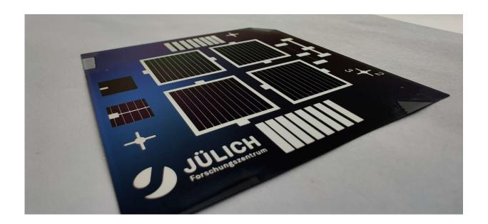
Prototype of the solar cells in laboratory size (TPC - Transparent Passivating Contact). Four solar cells, each measuring four square centimeters, can be seen on the silicon wafer, each of which is contacted and framed with screen-printed silver contacts. Credit: Forschungszentrum Jülich
