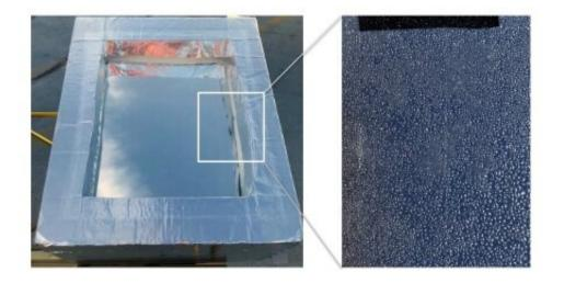
On the left, a look at the condenser unit. On the right, a closeup view of the water the unit is shedding. Credit: Ming Zhou, UW-Madison
