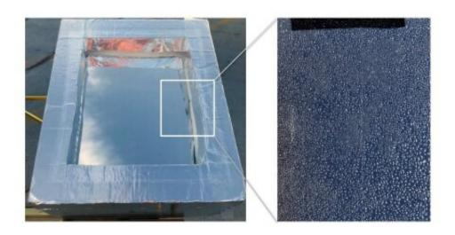
On the left, a look at the condenser unit. On the right, a closeup view of the water the unit is shedding. Credit: Ming Zhou, UW-Madison
