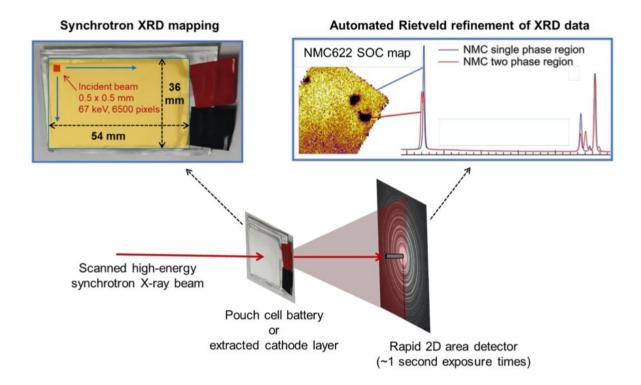
A schematic of the high-energy x-ray powder diffraction setup. Using automated software, the team mapped the battery state of charge (SOC) based on the diffraction data they collected for thousands of points across the battery. Credit: Brookhaven National Laboratory
