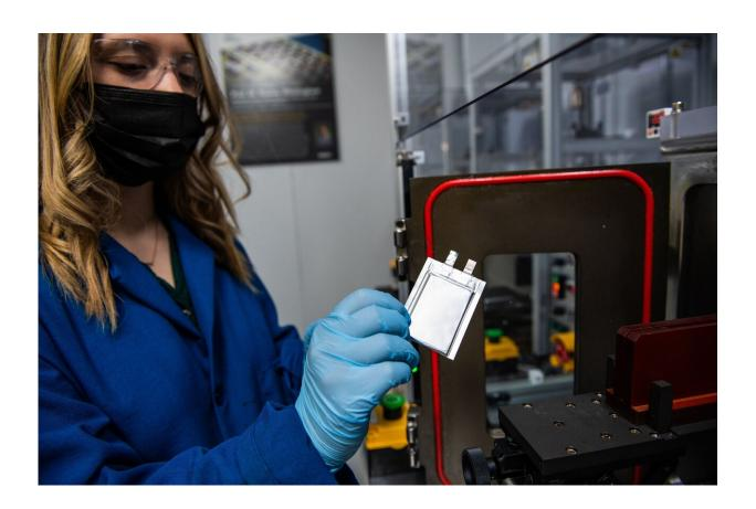
Cassidy Anderson, a PNNL post-bachelor intern and Battery500 Consortium team member, holds a pouch cell battery in PNNL's Advanced Battery Facility. The battery is enclosed in a polymer-based pouch containing an aluminum barrier layer to keep it safely sealed in an air-free environment. Credit: Pacific Northwest National Laboratory.
