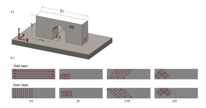
The researchers tested four different printing patterns, with the lasers either melting the powdered metal back and forth continuously or in distinct square islands and either running parallel to the long side of the part or diagonal to it. Credit: Lawrence Livermore National Laboratory/M. Strantza
