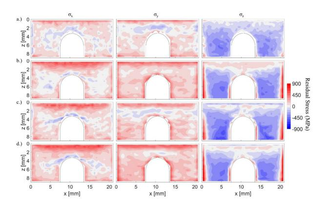
Using a laser-based method, researchers at NIST and other institutions 3D-printed four miniature metal bridges, each made with a different printing pattern (rows a-d). The team measured the levels of tension (red) and compression (blue) within the bridges in three different directions, identifying high levels of vertical tension along the edges of some specimens. Credit: Lawrence Livermore National Laboratory/M. Strantza
