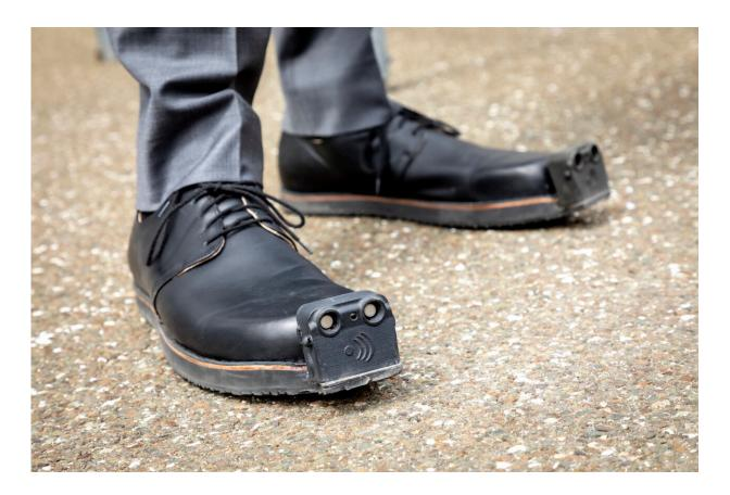
The Innomake shoe as it is now already available on the market. The ultrasonic sensor is attached to the toe of the shoe. In the future, a camera plus a processor running the algorithm will be integrated there. Credit: © Lunghammer - TU Graz
