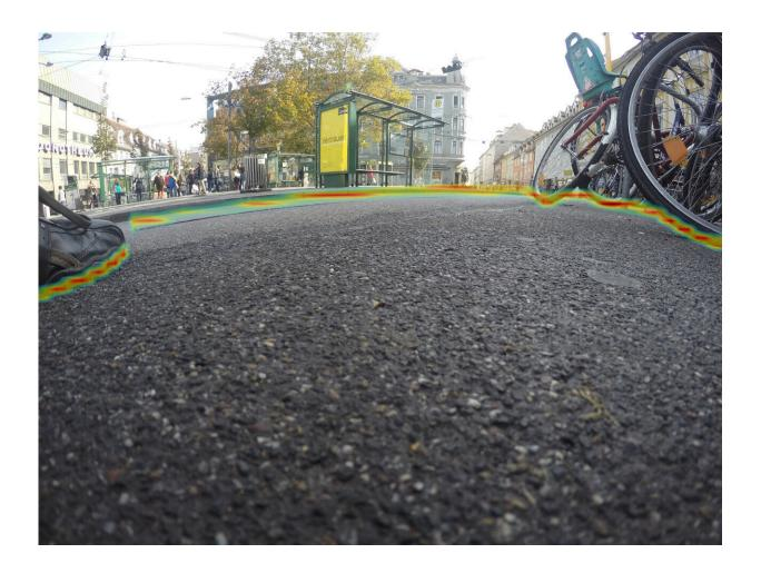
A camera shot from the perspective of shoes: the area that can be walked on without danger is delimited by color, recognized and interpreted by the image recognition algorithm of TU Graz. Credit: © TU Graz
