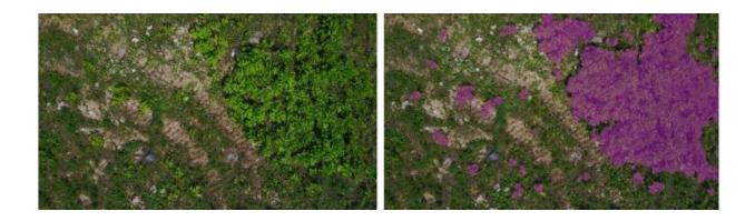
The input image (left) and the output image (right), processed by the fully convolutional neural network. Credit: Skoltech
