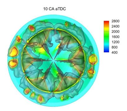
Argonne researchers used supercomputers to optimize the design of piston bowls in heavy-duty engines for Caterpillar Inc. The top designs reduced fuel consumption and soot formation, and others had potential to reduce NOx. Credit: Chao Xu/Argonne National Laboratory
