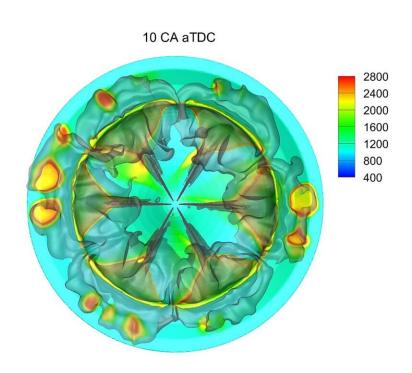
Argonne researchers used supercomputers to optimize the design of piston bowls in heavy-duty engines for Caterpillar Inc. The top designs reduced fuel consumption and soot formation, and others had potential to reduce NOx. Credit: Chao Xu/Argonne National Laboratory
