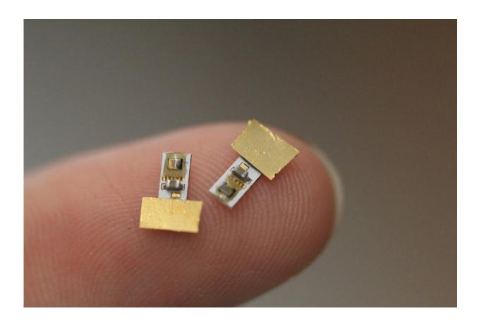
A new version of wireless implants developed at Rice University allows for multiple stimulators, as seen here, to be programmed and magnetically powered from a single transmitter outside the body. The implants could be used to treat spinal cord injuries or as pacemakers. Credit: Secure and Intelligent Micro-Systems Lab/Rice University
