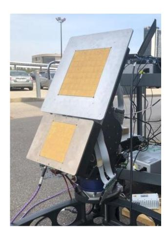
Receiver (top) and transmitter antennas developed by Waterloo Engineering researchers are shown during recent testing. Credit: University of Waterloo
