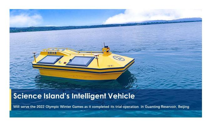
A water quality monitoring unmanned surface vehicle helps to improve the reservoir water environment. Credit: Yu Daoyang
