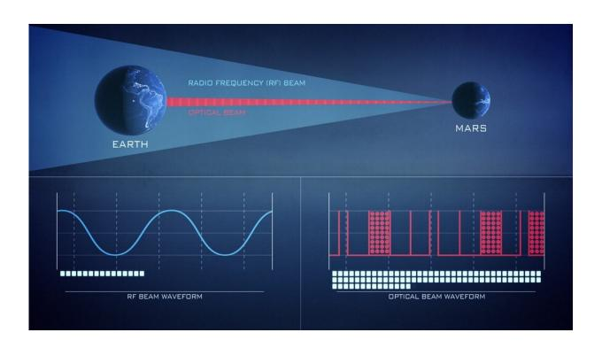
Graphic representation of the difference in data rates between radio and laser communications. Credit: NASA
