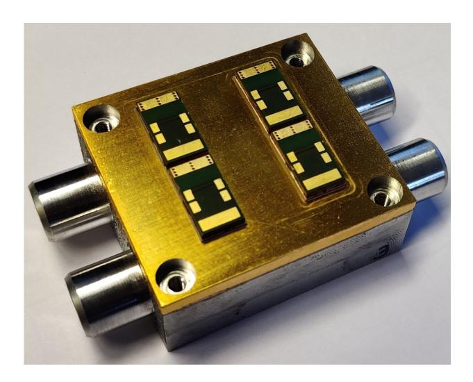
Well cooled and efficient – power inverters for Porsche power trains. Credit: Fraunhofer-Gesellschaft
