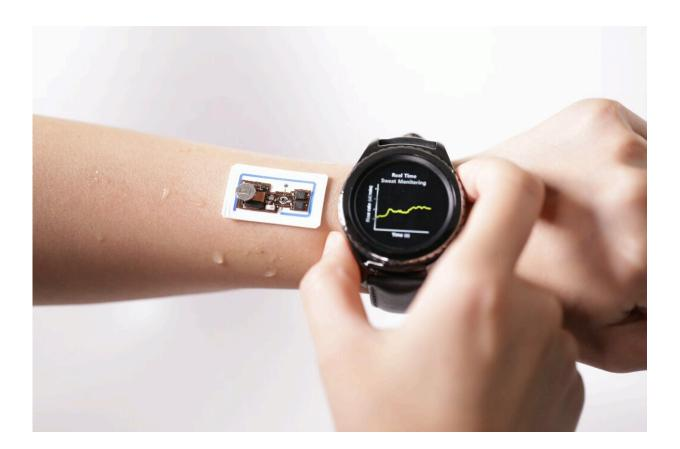
The electronic wireless system that softly interfaces to the skin to analyze the dynamics and chemistry of sweat released during physical exertion. Credit: Kwon et al.
