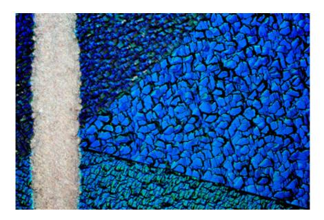
Figure 1: A light micrograph of a conventional photovoltaic cell based on polycrystalline silicon (blue crystals). Such solar cells use the photovoltaic effect to convert light into electricity. Photovoltaic devices based on the bulk photovoltaic effect could overcome some of the limitations of conventional devices. Credit: Antonio Romero/Science Photo Library
