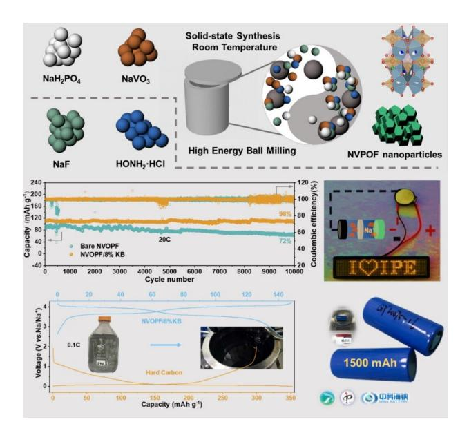
The electrochemical performance of sodium vanadium fluorophosphate
