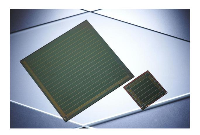
An innovative combination of processes enables the interconnection of cells to form modules with nearly no losses. (Photo: Amadeus Bramsiepe, KIT) Credit: Amadeus Bramsiepe, KIT
