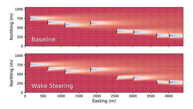
Illustration of wake steering for an example wind plant. Wind turbines are misaligned with the wind to redirect their wakes away from downstream turbines. Blue regions indicate lower wind speeds caused by wakes. Credit: Eric Simley, NREL
