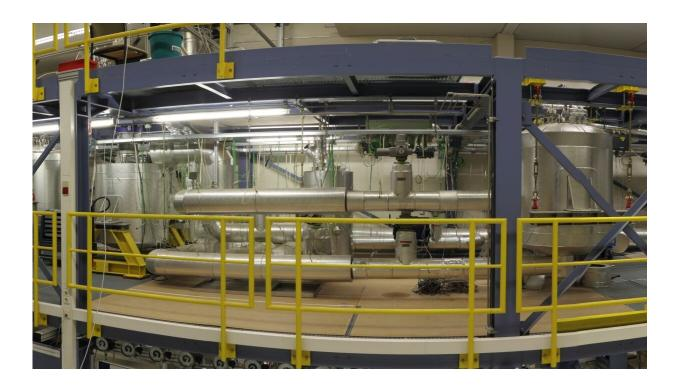
Within the framework of KIT's LIMELISA project, components for large-scale thermal storage systems are tested in a liquid metal circuit. Credit: Karsten Litfin, KIT
