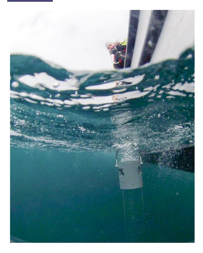
Maren Thu, from the Trondheim Biological Station, uses a Plexiglas water sampler, designed by NTNU researchers and built at the university. The design
