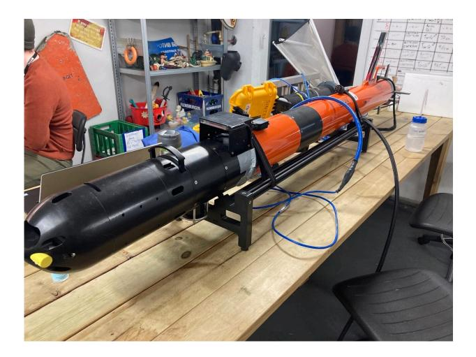
The star of the show: The lightweight autonomous underwater vehicle on a workbench, before deployment. Credit: Annecken Nøland
