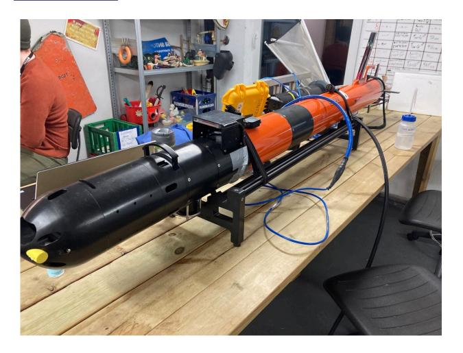
The star of the show: The lightweight autonomous underwater vehicle on a workbench, before deployment. Credit: Annecken Nøland
