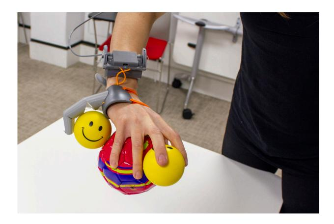
Using the 'Third Thumb' to complete one of the training tasks, of holding multiple balls with one hand. Credit: Dani Clode
