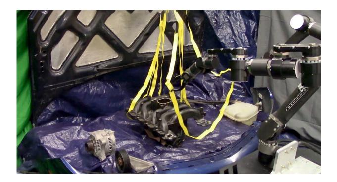
A robot performs the difficult to model task of manipulating straps without tangling them around a mock car engine in the Autonomous Robotic Manipulation Lab. Credit: Peter Mitrano
