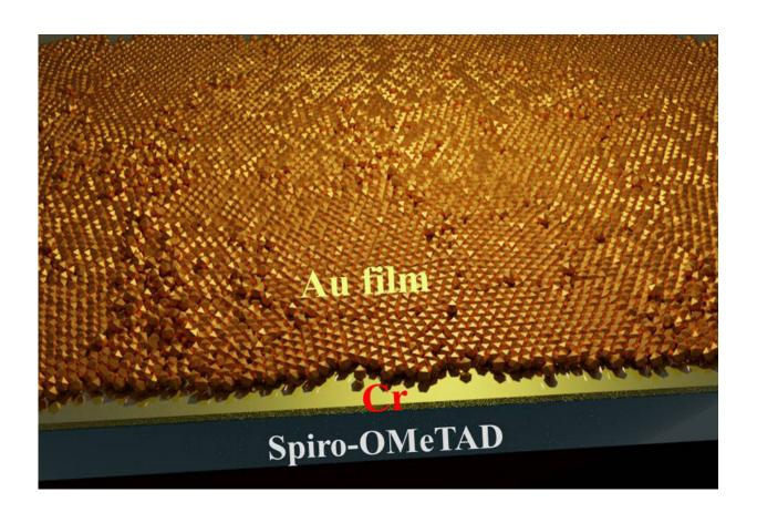
Scientists found using a chromium seed layer allowed them to grow ultrathin gold film that serves as a transparent electrode with good conductivity for perovskite solar cells. Credit: Penn State
