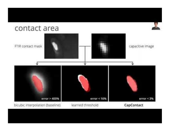
The "CapContact" method can localize the touches by fingers on the touchscreens of mobile phones and tablets much more accurately than current industry-wide technology. (Video: CHI/SIPLAP)
