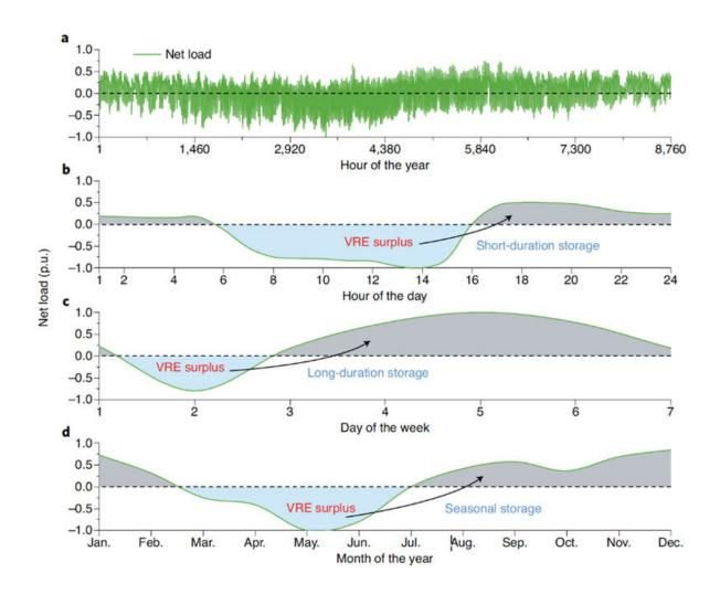
This graph of multiscale energy storage needs for a hypothetical 95% carbon-free power system assumes 28.4% wind and 51.5% solar PV energy share. Energy storage requirements are shown for (a) Hourly net load over the course of a year; (b) Hourly net load for a given day; (c) Total daily net load for a given
