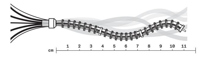
The "tendon-driven" continuum robots depicted here are, in real life, about seven millimetres in diameter and are built in sections that can range in length from 15 to 70 millimetres. Other models can be even narrower. All exhibit a tentacle-like motion. Credit: Colin Hayes
