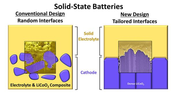
Illustration of a conventional solid-state battery and the team's new highperformance design that contains tailored electrode-electrolyte interfaces. Credit: University of Illinois at Urbana-Champaign
