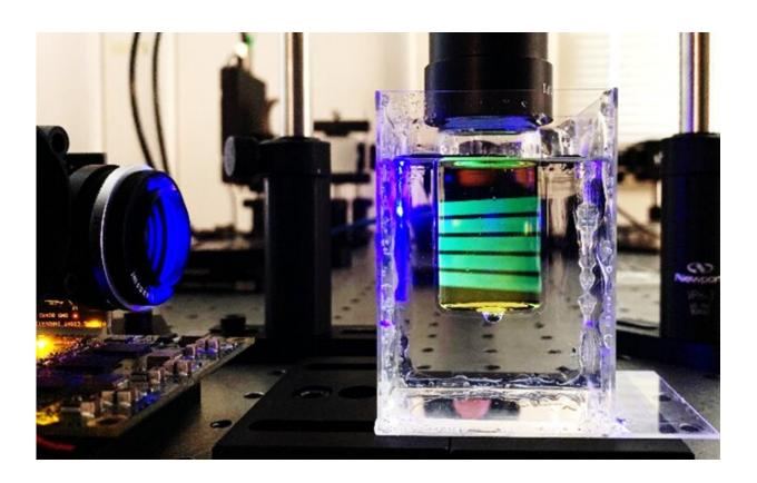
Now you see it, now you don't: tomographic printing using the goopy index bath. The green light in the vial is fluorescence – a by-product of the 3D printing process that conveniently highlights the path of light in the vial. Credit: University of Waterloo
