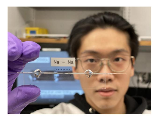
Bingyuan Ma holding a transparent capillary cell. Bai's Lab at the McKelvey School of Engineering is the only one in the world with such diagnostic cells. Credit: Peng Bai Lab
