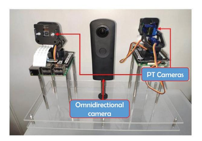
Researchers from Shibaura Institute of Technology, Japan design a dual camerabased platform employing an omnidirectional camera for target detection and a separate camera for its high-resolution capture and report an overall improved performance, opening doors to potential applications in security systems. Credit: Shibaura Institute of Technology, Japan
