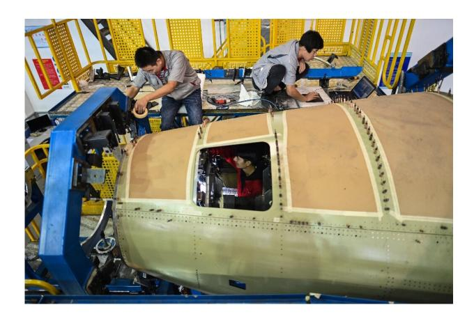
Employees work on an aft fuselage section of a C919.
