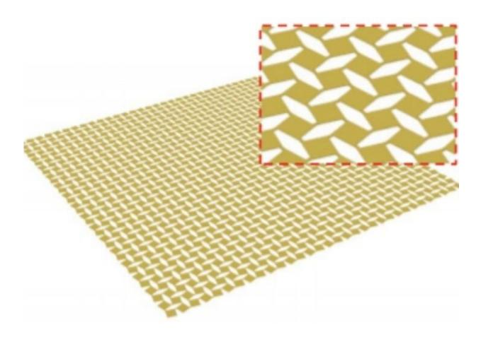
Schematic of a biaxially stretched kirigami sheet. Credit: University of Houston
