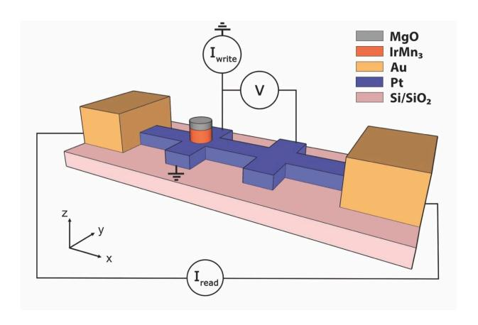
Schematic representation of the device, showing the current sources and the nanovolt meter (V)connections for one of the switching experiments. Credit: Northwestern University and the University of Messina
