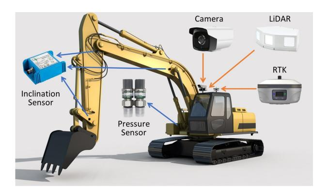
LiDAR, cameras, and proprioceptive sensors are mounted on the excavator to perceive the 3D environment. Credit: Baidu Research
