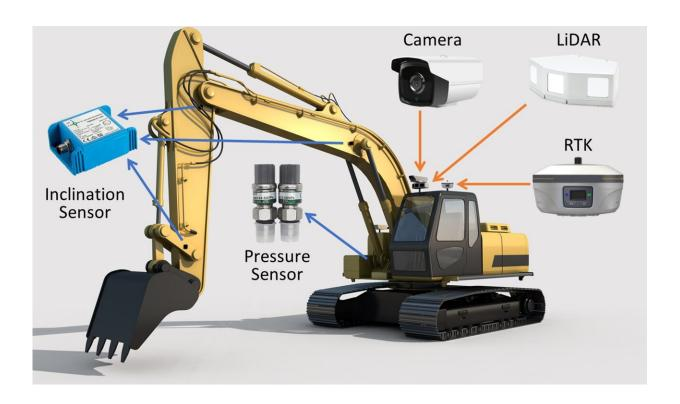
LiDAR, cameras, and proprioceptive sensors are mounted on the excavator to perceive the 3D environment. Credit: Baidu Research
