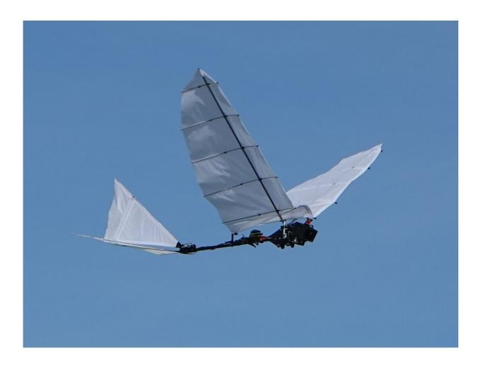
The GRIFFIN project is seeking to create prototypes of highly autonomous, ultralightweight robot birds. Credit: GRVC Robotics Lab
