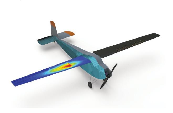
MIT researchers propose a formal mathematical representation of a digital twin and its associated physical asset, and demonstrate how their formulation naturally integrates data, predictive models, and decision-making to enable the creation of a structural digital twin for a self-aware unpiloted aerial vehicle that dynamically replans its mission in response to in-flight structural damage. Credit: Massachusetts Institute of Technology
