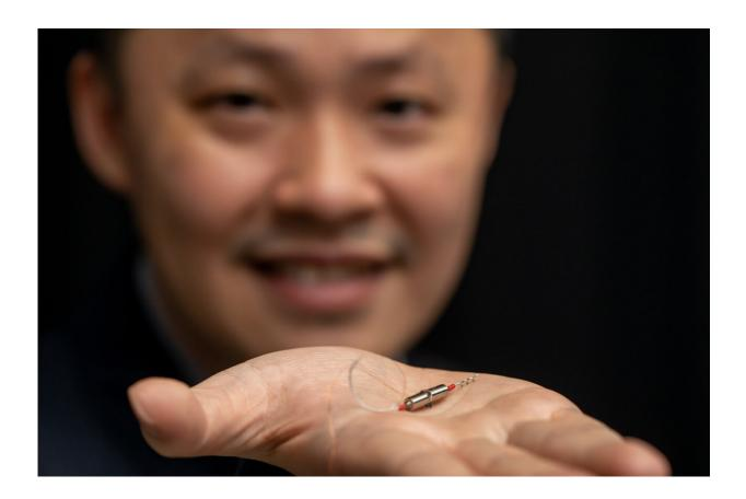
The bio-inspired robot consists of three parts like the ray sperm: a spiral head made of rigid iron wire, a helical tail made of soft cotton wire, and two motors as the midpiece for the energy supply. Credit: City University of Hong Kong
