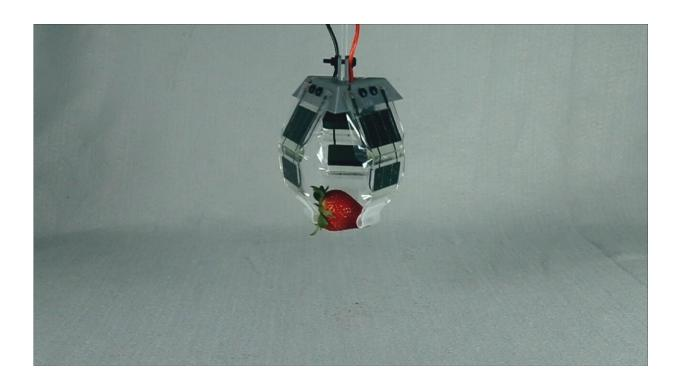
A robotic gripper based on SES joints grabs a strawberry without damaging it. Credit: MPI for Intelligent Systems and University of Colorado Boulder
