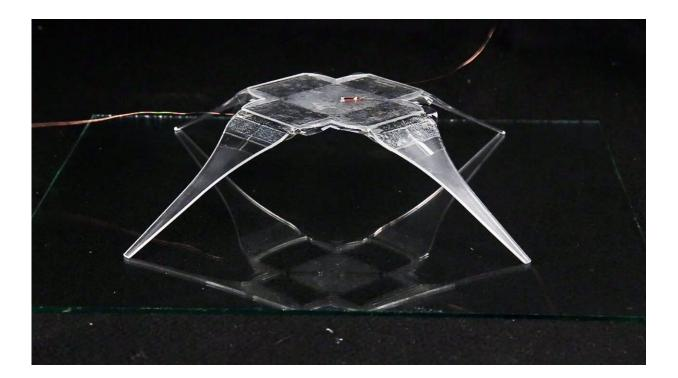
SES joints can be combined to create different types of robotic structures such as this four-legged robot that looks like a spider. Credit: MPI for Intelligent Systems and University of Colorado Boulder
