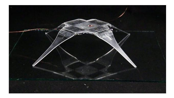
SES joints can be combined to create different types of robotic structures such as this four-legged robot that looks like a spider. Credit: MPI for Intelligent Systems and University of Colorado Boulder
