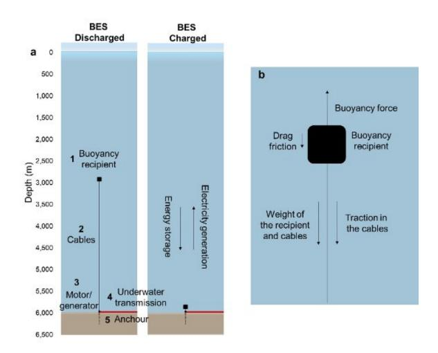
Buoyancy Energy Storage, (a) the system and main components, (b) forces exerted in the buoyancy recipient. Credit: International Institute for Applied Systems Analysis
