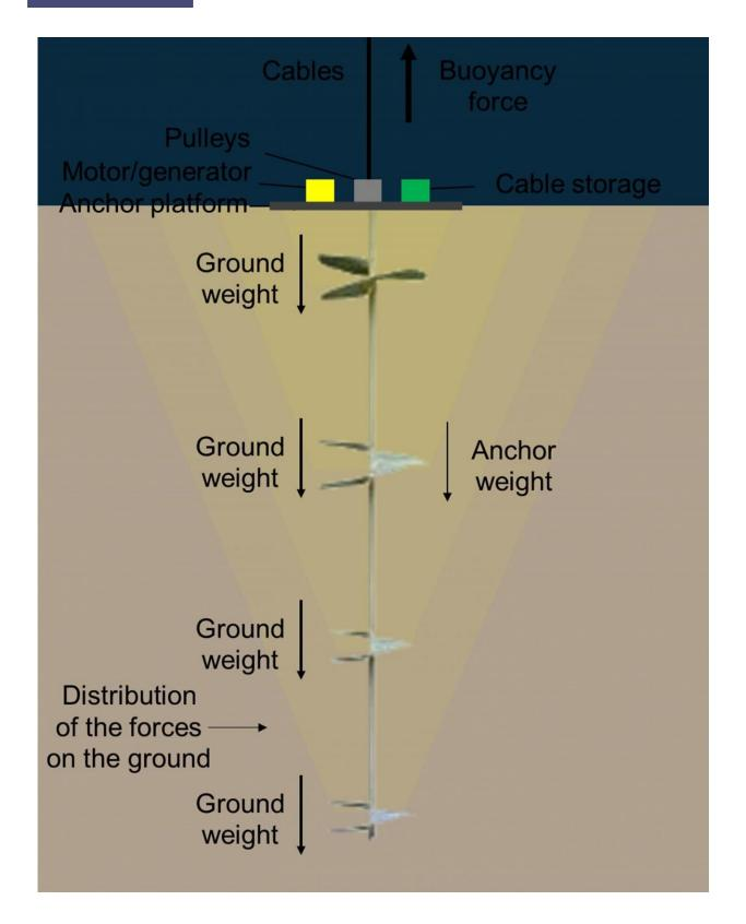
Proposed Buoyancy Energy Storage System. Credit: Hunt et al. (2021)
