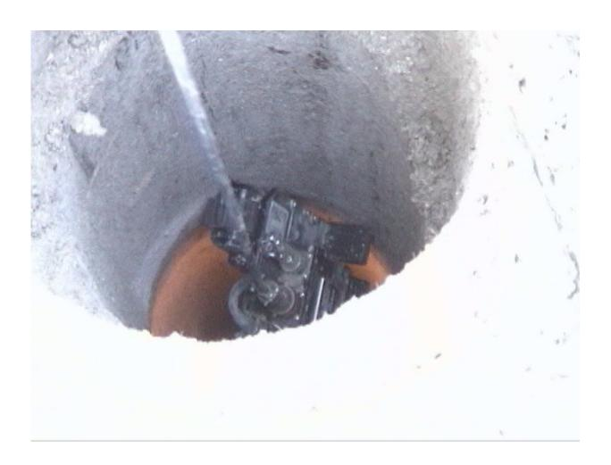
An Inuktun crawling robot being lowered into a hole at the World Trade Center site in 2001. Credit: Center for Robot-Assisted Search and Rescue
