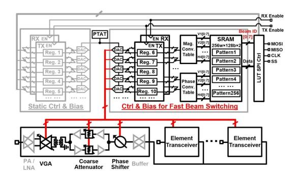
Large volume SRAM and lookup table are used for supporting 256 beam settings. The mechanism supports fast switching in transmit (TX) and receive (RX) mode with direct external TX/RX enable pins. Credit: 2021 Symposia on VLSI Technology and Circuits
