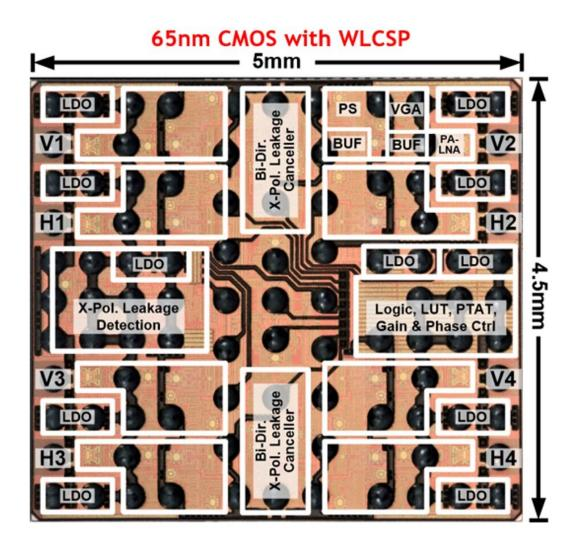
The proposed phased-array transceiver is fabricated using a 65-nm CMOS process and packaged with wafer-level chip-scale package. It is configured in an area as small as  $5 \times 4.5$  mm. Credit: 2021 Symposia on VLSI Technology and Circuits
