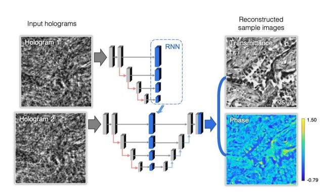
UCLA researchers demonstrated holographic imaging using recurrent neural networks (RNN). A human lung tissue section is imaged with faster and better hologram reconstruction. Credit: UCLA Engineering Institute for Technology Advancement
