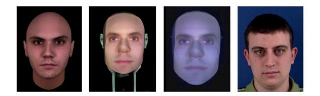
The different types of embodiments used in the experiment. From left to right: a virtual agent, a physical Furhat robot and a video recording of the Furhat robot. The rightmost picture shows the video of a human used as control condition. Credit: Perugia et al.
