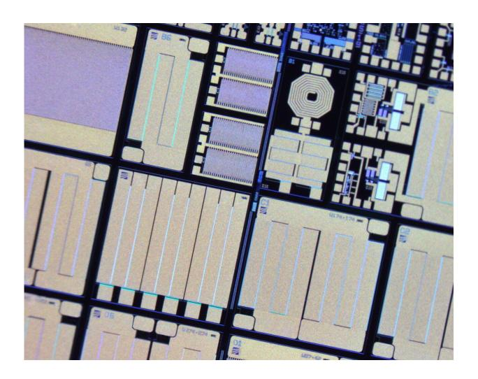
Fraunhofer IAF's innovative GaN-on-Si chip designs offer efficient and highly compact components for future low-voltage applications. Credit: Fraunhofer IAF
