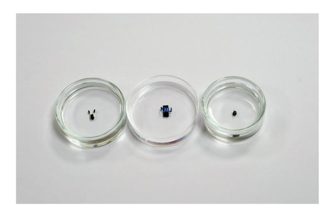
The NTU millimetre-sized robots measure about the size of a grain of rice and can be controlled using magnetic fields. Credit: Nanyang Technological University
