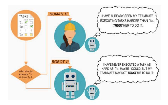
A team formed by a human and a robot that must collaborate sequentially executing tasks. Each task must be executed by one of the agents. The bidirectional trust model can be used for predicting the human's natural trust in a robot to execute a task, and for the robot to determine its artificial trust in the human to execute a task. Credit: Azevedo-Sa et al.
