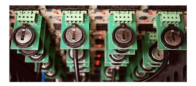
Prototype lithium metal batteries with carbon nanomembrane modified separators being tested at Wayne State University. Credit: Sathish Rajendran/Wayne State University
