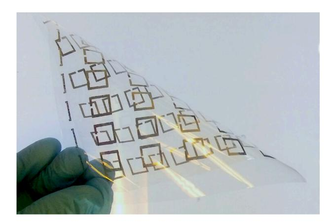
A thin film polymer tunes the properties of an inkjet printed array of small microwave resonators. The composite device can be tuned to capture or transmit different wavelengths of microwave energy. Credit: Fio Omenetto, Tufts University
