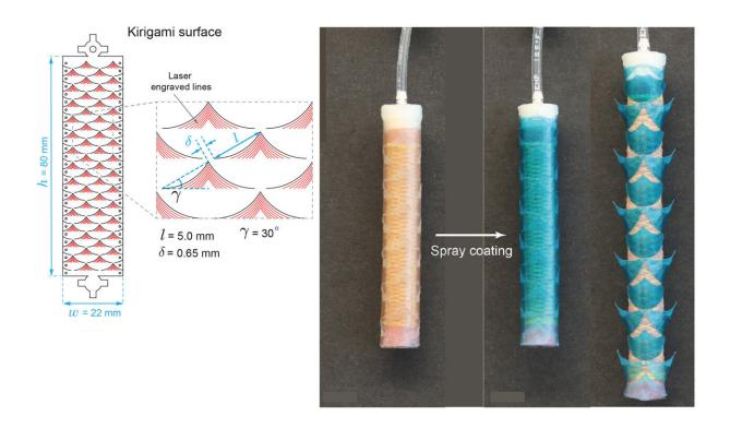
The device has two key elements -- a soft, stretchy tube made of silicone-based rubber, and a plastic coating etched with needles that pop up when the tube is stretched. Credit: MIT
